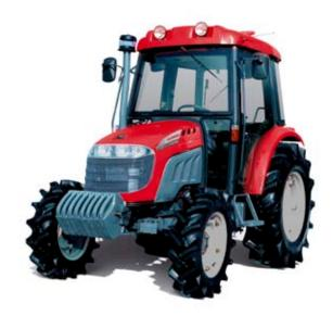
Available with either ROPS or cab, the X10.55 series tractor offers a comfortable and ergonomic driving position. The stylish, sloping engine hood design and the rounded fender shape make for outstanding all-round visibility and excellent manoeuvrability. The iso-mounted platform is large and roomy. The cab is fitted with heating, air-conditioning, radio, roof hatch and four work lights. A deluxe seat, along with the ergonomically-arranged controls, further enhances the operator comfort.
