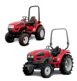
From the smallest X10.25 to the largest X10.35, all models in this range are specially designed to perform light farm tasks as well as lawn and landscape maintenance jobs. They are powered by Tier 3-compliant, 3-cylinder, water-cooled diesel engines delivering 22, 28 and 34 hp, respectively.
